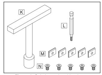
Figure 6. Spiral cutterhead hardware.
